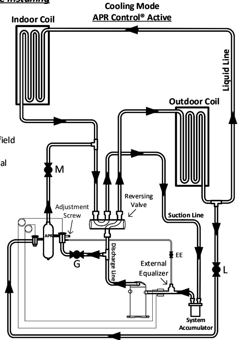
Isolation valves M-G-L to be field supplied and installed
