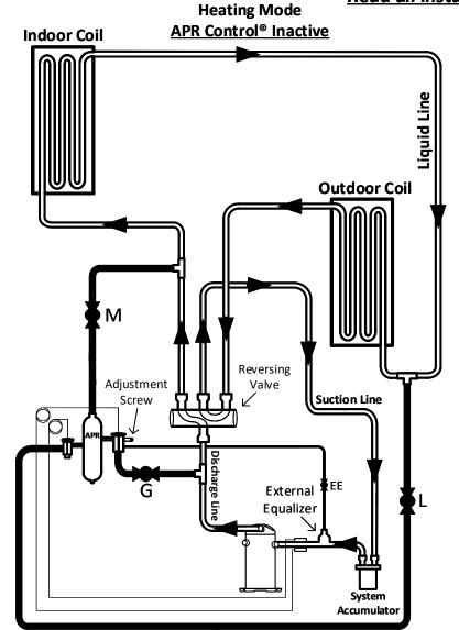
Isolation valves M-G-L to be field supplied and installed \*EE optional to provide total isolation
