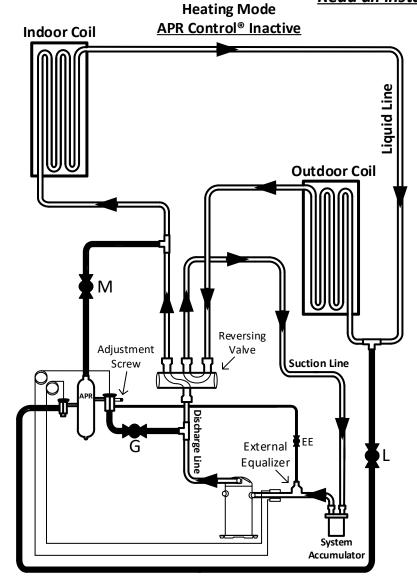
Isolation valves M-G-L to be field supplied and installed \*EE optional to provide total isolation
